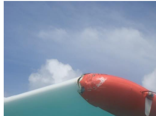
Figure 12: Damage left wingtip fairing
