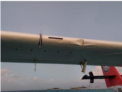
Figure 11: Damages to Right Wing
